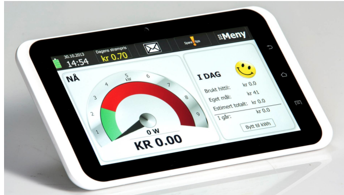
Figure 1.2: The eWave display being offered to Fredrikstad Energi's customers. The display is 7 inches across, and is based on the Android platform (photo by Odin Media).
