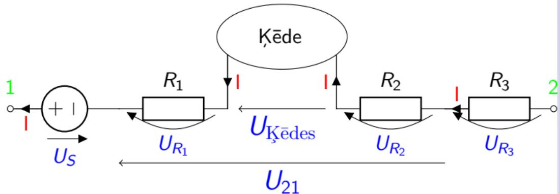
$$I = \frac{\varphi_1 - \varphi_2 + U_{\text{Kēdes}} + U_S}{R_1 + R_2 + R_3}$$
