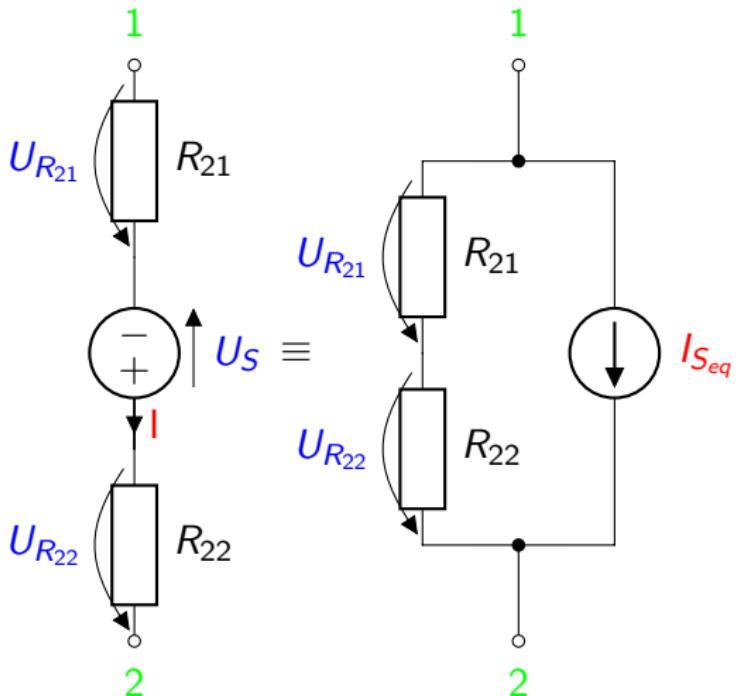
$$I_{S_{eq}} = \frac{U_s}{R_{21} + R_{22}} = U_s \cdot G_2$$
