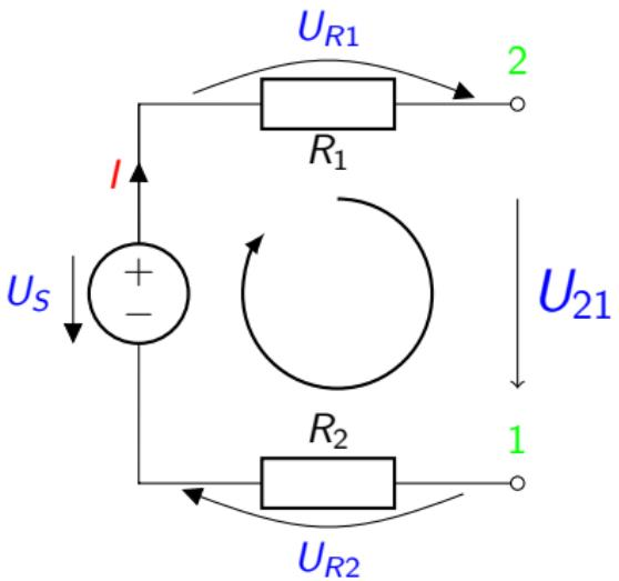
$$U_{21} = \varphi_2 - \varphi_1 , \quad U_{R_1} = I \cdot R_1 ; \quad U_{R_2} = I \cdot R_2$$
