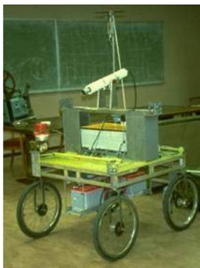
Figura 1.1: Robot Stanford Cart.
